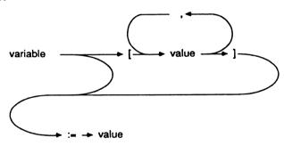
Imagine you are an engine that can only go forward. Start at the beginning of the diagram at the word VARIABLE. Every time you see a branch, you can take it or not. Every time you encounter a symbol or word that is not part of the tracks, except for the arrows which are part of the tracks, you collect that item. All symbols and upper case words are collected exactly as they are shown in the diagram. Lower case words are further explained elsewhere, such as the section on DEFINITIONS.
