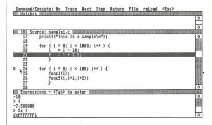
Set a breakpoint on the line shown above (on line 24). Do this by clicking with the mouse anywhere on the desired line. Notice the indicator in the left most column.
