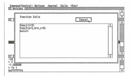
Choose **Step** until the current line is on the "sprintf()" in the function "func1()". Then choose **Calls**, also from the **Control** menu. This shows the current function calling order and the parameters of each. Try this when "main()" calls "func2()" which calls "func1()."
