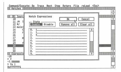
Open the **Watch** dialog. Go back to the main menu with the **Execute**, or type **Ctl>-W** directly from the **Execute** menu. Enter the three variables as shown above. Make sure the "Enable" item is selected. Click "Ok" when done.
