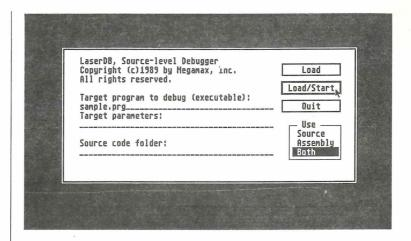
When the Startup dialog appears, just press <Return> or click on "Load/Start". The configuration file has already been set for this example. The program being debugged is SAMPLE.PRG. It was compiled from two source files called SAMPLE1.C and SAMPLE2.C. When "Load/Start" is pressed, the executable and the source will be loaded, and a **Step** will be executed which will step from the initialization code *into* the function "main()".
