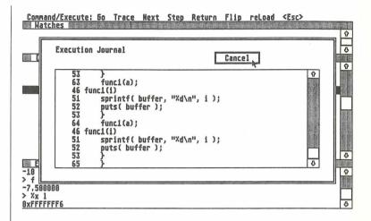
Choose **Journal** from the **Control** menu. <Ctl>-J is the shortcut for this command. This shows all source lines traced or stepped. In the assembly mode, disassembled instructions are shown here.
