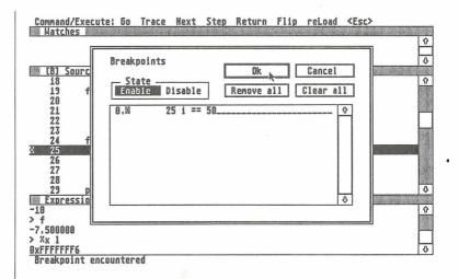
Set a breakpoint on the line shown above and choose Go or Next until the breakpoint is encountered. Now open the Breaks dialog by choosing it from the main menu, or by typing <Ctl>-B. The breakpoint on line 25 is the one just set. Enter the break expression shown above. Close the dialog with "Ok". Make sure "i" is less then 50. If it is greater than 50, enter the following expression using the <Tab> command:
