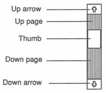
Clicking on an arrow moves the window over it's contents in the indicated direction by one line. Clicking in the page scroll area moves the window by one page. The thumb may be dragged to reposition the window over any part of it's contents.
