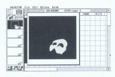
DA'S VECTOR can be used to generate film sequences of up to 10,000 single pictures. You begin with a blank ("unexposed") film. You do not need, however, to "expose" all pictures. Depending on the type of animation, a few "keyframes" are often sufficient. All in-
