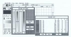
internally with 16.7 million colours. You can use two different colour systems: the RGB and the CMYK systems. In principle, both systems can be converted into each other, especially if you
