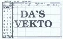
submenu consisting of four basic functions and a character selector box in which the characters of the current font are displayed (over several "pages" accessed by the arrow icons). This display is not just for viewing since you can click on the characters in text entry mode and insert them into the text that way; this gives you access to all the special characters. If you have not loaded any particular font (see below), you see the (vectorised) system font.
