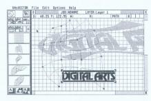
reshaped. Now you can "project" a graphic object onto this grid using the calculation function and thus realise virtually any kind of flexible reshaping of objects. This is quite difficult to describe in words; you should simply try it out for yourself and examine the predefined grids in the library. You will find this an intuitive method of flexible reshaping which allows you to forget about all the mathematical background and rules.
