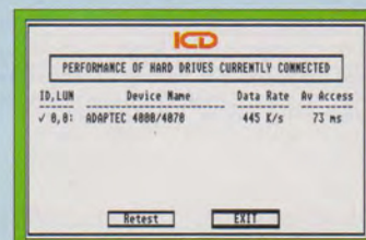
RateHD, one of the ICD utilities, testing an old Megafile 30 with the truly appalling access time of 73 milliseconds!
