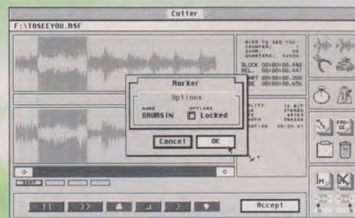
You can place and name up to 64 markers in a sample by dragging them into the waveform area.
