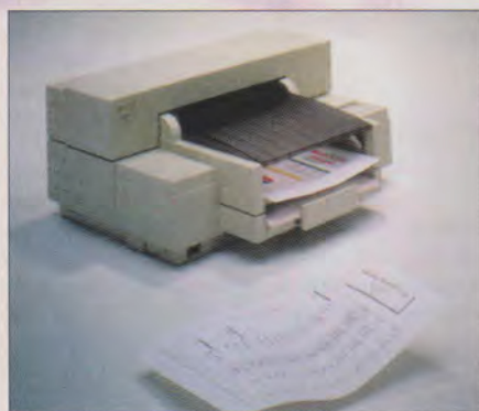
Hewlett-Packard's latest, the DeskJet 560c, has an improved resolution of 600 by 300 dots per inch.
