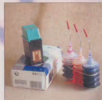
Close up of a tri-colour HP DeskJet 550c cartridge – three separate ink containers are used.
