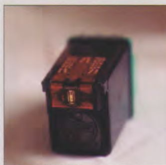
A close up of an inkjet head; note the small jets along the top of the unit.
