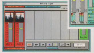
Figure 3: DigiTape has a fully configurable mixer section. Each channel may be used to monitor tape tracks or to control an effect module. Here, two tracks and two effect modules are installed.
