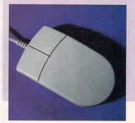
uses micro-switches for the buttons, making it much lighter and easier to click. Our mouse also has a much higher resolution - 280 dots per inch which means you need far less desk space and get much finer control.
