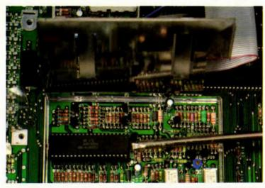
Note the video shifter chip's orientation before gently levering it out of the board. Bew very careful not to bend any of the legs. Once attached to the new board (picture seven), it must be re-located back here as it was.
