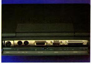
The power lead, RS 232 serial interface, parallel printer port, ASCII DMA port for external 3.5 floppy or hard disk and the allimportant sub-miniature MIDI in / MIDI out ports.
