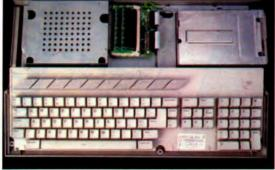
And here we are, with everything back in place. The SIMMs module nestles rather neatly between the disk drive and the power unit. It's a good idea to fix it here permanently with some handy adhesive pads.
