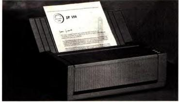
uite a different machine from the others in this group. If you sawed the print trays and control panel off an HP DeskJet you would end up with the JP150 – a slightly oversized grey shoe box based on the Hewlett Packard print engine.
