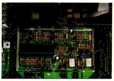
Open the lid of the box to reveal the video shifter chip. This has to be removed and re-fitted onto the board supplied (picture seven). Some video chips are soldered in and require de-soldering by a competent technician.
