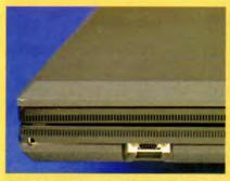
Sneakily tucked away is this connector, which is, suprisingly, destined for a second keyboard or an Atari mouse. Neither of these plug-ins have yet been sighted, but watch this space...
