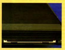
Behind yet another neat sliding cover lies a 120-pin extension bus providing direct access to the CPU. An optional 120-pin adapter will allow you to plug in existing ST cartridges or dongles. This means that the true compatibility of software across the ST range is not impaired – even with plug-in dongles.
