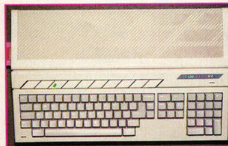
C-Lab's Mk 2 Falcon is aimed primarily at MIDI musicians and has been modified to facilitate direct-to-disk recording.
