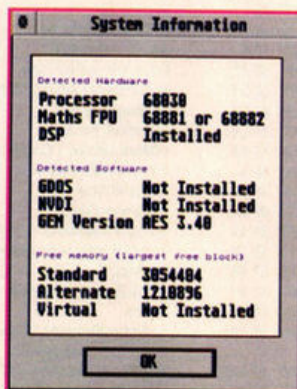
Positive Image detects hardware extras such as Alternate (TT) RAM, DSP and FPU, and will also create a swap file on hard disk drives.
