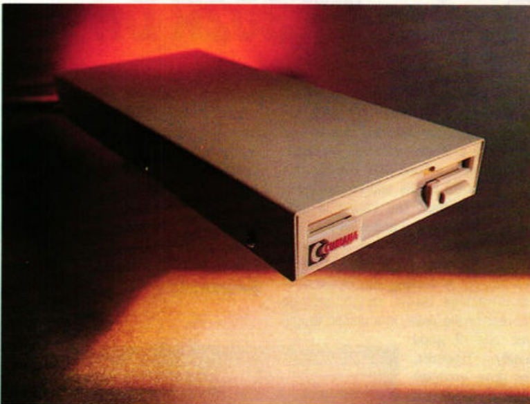
● The Cumana CSA 354 scores for its solid construction, good quality internal power supply unit and attention to detail – the correct fuse is included.
