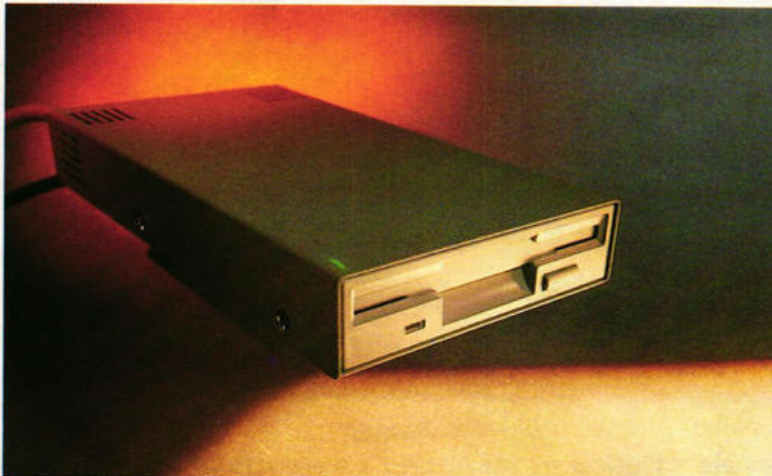
● The Power PC720E is virtually identical to the PC720 but draws its power from the ST's joystick port – a bit Heath Robinson, but it's cheap and it works effectively.
