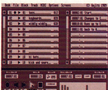
■ The cue sheet on the right enables any point within the piece to be dragged to either song position or locator marks
