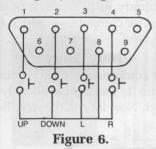
Each input line turns on or off 1 bit in memory location 54016. Both joysticks 1 and 2 are read from this location. Joystick 1 controls the first 4 bits of 54016, and joystick 2 the last 4 bits. Since inputs to logic circuits are always 1 unless connected to ground (logic 0), then PEEK(54016) should be 255 (11111111 in binary) when no joystick is present.
