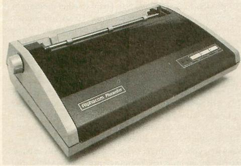
The **101** also features a 93-byte buffer, expandable to 4000 bytes. The printer offers selectable pitch and handles paper up to 13 inches wide. Diablo- and Qume-compatible print wheels are interchangeable on the **101**. There's also an Atari-compatible **101** available, packaged with a serial port adapter and instructions for Atari users.
