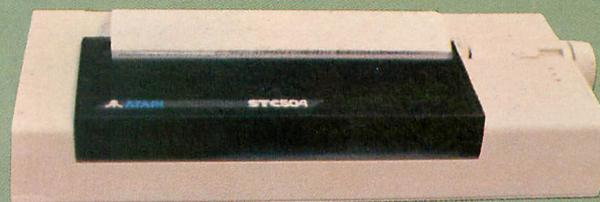
Above: the STC 504, the new dot matrix, non-impact, color printer. Below: the SDM 121, Atari's daisy wheel letter quality printer.
