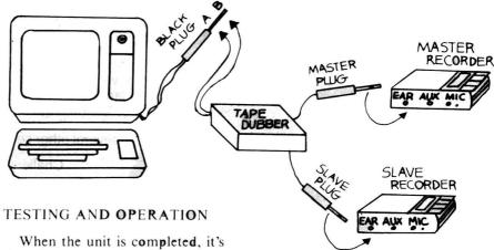
When the unit is completed, it's time for some testing. Plug the 'Master' plug into the ear jack of your master recorder (the one you normally use). Connect the two alligator clips to the black plug from the computer. Be sure that clip B connects to the tip terminal and clip A connects to the body terminal. Also be sure these two clips are not touching. With the power on, load tapes as usual. Note: The two gray plugs from the computer connect normally.
