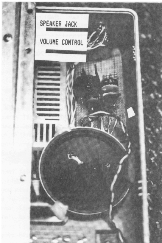
PHOTO #1 SHOWING LOCATION OF SPEAKER JACK, VOLUME CONTROL, AMPLIFIER BOARD AND SPEAKER
