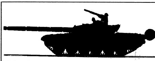
T-72 Main Battle Tank With Long Range Fuel Tanks
