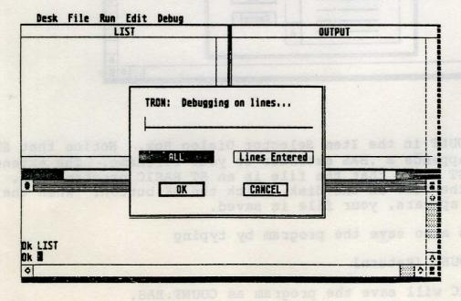
The Tron option displays the program's line number in the Command Window as each program line is executed.
