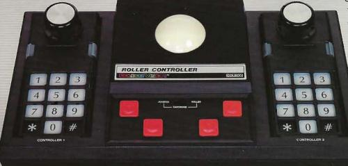
The MODE SWITCH lets players select the appropriate play mode to suit the cartridge, either ROLLER or JOYSTICK. Hand Controller Wells for ColecoVision® joystick controllers are located on each side of the Roller Controller Console. The ROLLER CONTROLLER can also be sued with most ColecoVision® cartridges that can be played with a standard hand controller.
