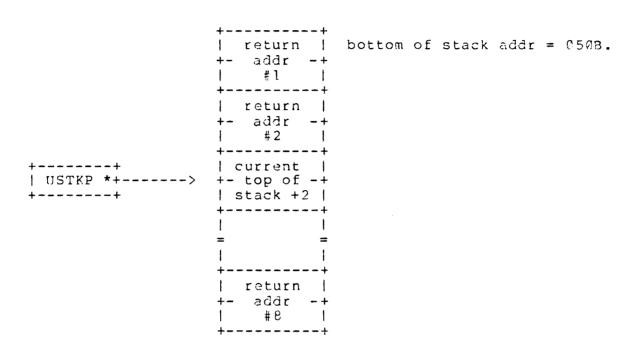
The Use stack pointer USTKP [0090] is a single byte quantity which contains an index value to the word beyond the current top of stack (next available free word). For the case of an empty stack USTKF ontains 0 and is then incremented by 2 for every item added to the stack (Use command) and decremented by 2 for every item deleted from the stack (End command).
