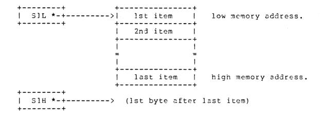
When the program list is empty, SlL and SlH both point to the first usable byte at the beginning of the free memory region. The value of SlL is established from O.S. variable MEMLO [02E7] at power-up time and is not altered thereafter.
