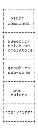
Each segment in the table contains one or more name entries plus a segment terminator byte of zero. A single name entry is shown below:
