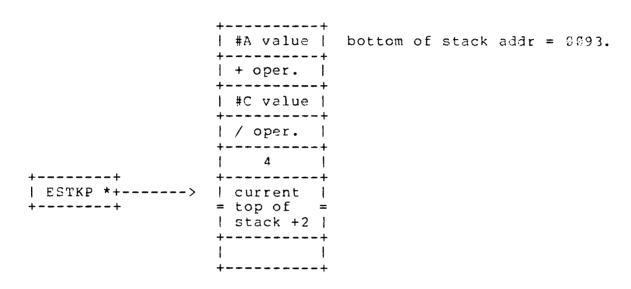
The expression stack pointer ESTKP [0091] is a single byte quantity which contains an index value to the word beyond the current top of stack (next available free word). For the case of an empty stack ESTKP contains 0 and is then incremented by 2 for every item added to the stack and decremented by 2 for every item deleted from the stack.
