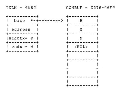
When PILOT is in run mode, the INLN pointer points to program statements in the program storage area (instead of COMBUF). In that case the base address points to the beginning of the statement allocation and the start index contains a value of 6 which offsets the overhead bytes. See section 4.3 for the format of the program statement storage.
