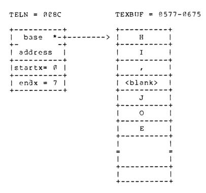
Although TEXBUF could in theory be dynamically assigned, there is code within the interpreter which accesses the buffer by name rather than using the pointer TELN, thus making dynamic assignment impossible (without coding changes to the interpreter).
