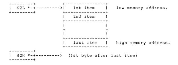
When the string list is empty, S2L and S2H both point to the first unusable byte at the end of memory. The value of S2H is established from O.S. variable MEMTOP [02E5] at power-up time and is readjusted whenever there is a change in the screen mode due to a Graphics command execution.
