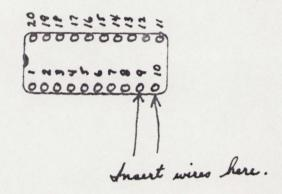
Now re-insert the PAL chip (along with the wires) making certain that you don't bend any of its pins, that all pins are in the socket and that the notched end of the PAL chip is toward the left! Make sure that chip is firmly seated all the way into its socket and that the O.S.P.S. wires are in their proper holes and that the bare wire ends are not shorting across any other pins or touching anything metal.
