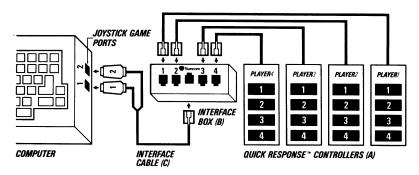
The next step is to connect the PQ Interface Box **(B)** to the computer. There are five connector jacks on the interface; four are numbered for connecting the four Quick Response Controllers. In the center of the interface box is a fifth jack, located under the
