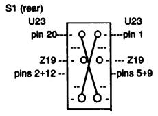
Note: where the wires cross in the middle, they are NOT connected. Make the connection from the switch to U23 on the rear of the mother-board.
