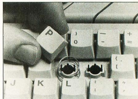
**Does anybody remember the Atari 400?** This kid brother of the classic Atari 800 was known for its small size and its use of a flat, plastic keyboard that offered little to no tactile feedback. The keyboard on the ST feels similar to the 400's, because underneath those white sculptured keys, it too possesses a flat keyboard.
