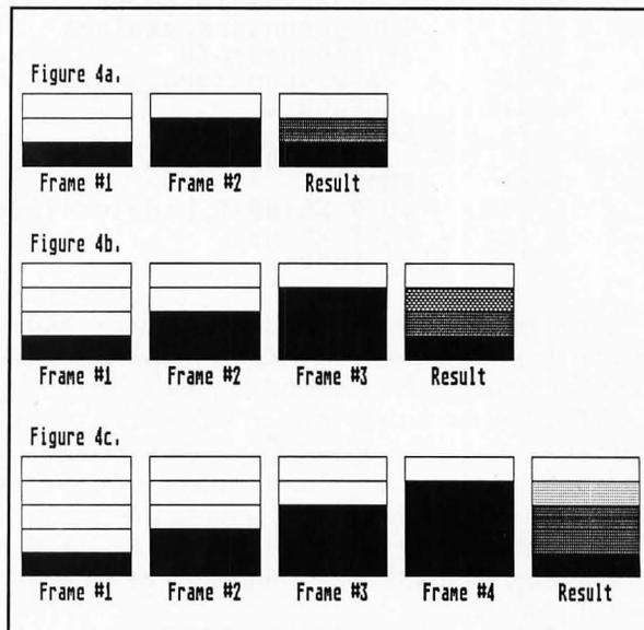
with the middle third alternating. By merely adding extra frames to the sequence as shown in Figures 4B and 4C, we can generate three and four visible brightness levels.
