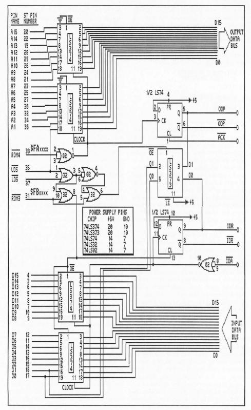
With 16 address lines, we could address up to 64K in our circuits. The 68000 actually has 24 address lines however, and can address up to 16 megabytes!
