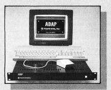
Sampling and SMPTE hardware: The revolutionary ADAP SoundRack (Analog to Digital Audio Processor) takes full advantage of the speed and memory of the ATARI 1040ST. The "ADAP" is a hardware/software peripheral for the ST that allows music and broadcast professionals to sample 20 seconds at 44.1 khz with 16 bit resolution. Full //IDI compatability is implemented. System is upgradeable to direct to hard disk stereo digital mastering and SMPTE interlock.
