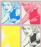
■ Any colour picture in Postscript is made up from four films, supplying the cyan, magenta, yellow and black components of the image.
