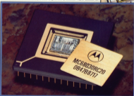
Motorola's 68000 microprocessor: the most recent member of the 68K family. 'On-chip' is often described as a mainframe on a chip. The processor boasts a clock rate of 25MHz, instruction and data caches, parallel processing facilities. Barely 10¢ (a result of spending up information transmission from main chip) and 68K series compatibility. 4-800-P you want too!
