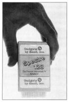
The slender Spectre cartridge shell is the same as the one used in Deskcart. You can leave it plugged in all the time, since it is active only when you run the Spectre software.
