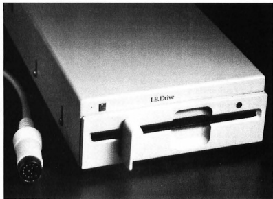
The I.B. 5¼-inch drive has a storage capacity of 360K and is invaluable when using pc-ditto.
