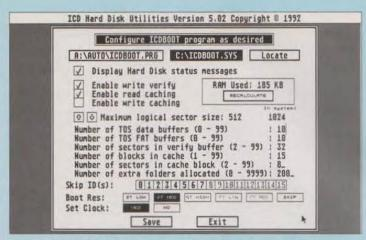
Setting the ICD disk cache supplied with ICD hard drives.
