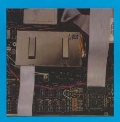
Having rounded the edge of the box where the cable is going to go through, close and seal the lid of the Shifter box. Now replace the screen and run the cables through to the top and out to the side of the power supply. This is probably the most awkward stage of the whole procedure and may take a couple of attempts to get right!
