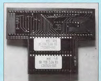
The TOS 2.06 upgrade board from COMPO.
