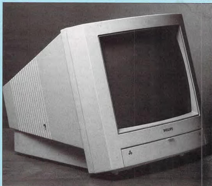
The Philips CM8833 Mk II features stereo sound from the STE.
