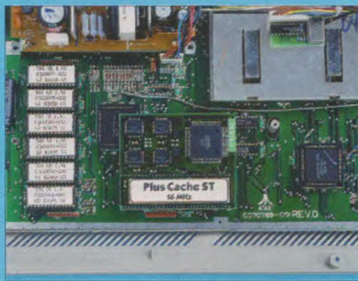
The Plus Cache board in place. The board must be set at an angle if it is to fit comfortably under the keyboard.
