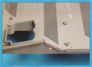
Drill a hole in the case of the ST for the switch. The diameter for this should be six millimetres.
