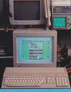
When the power supply, drive and keyboard are replaced, it looks just like any other ST, but it has a secret. Connect all of the leads, place the switching software in the drive and switch on. You now have the choice of TOS 1.02 or 2.06.
