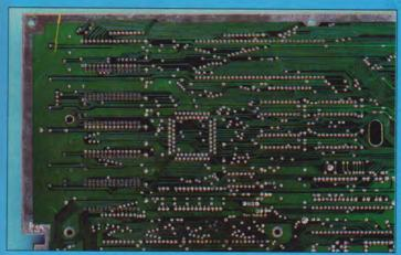
Turn the board over and identify the 68000 from the back. Place a piece of insulating tape directly on the board under where the upgrade will go. This will reduce prevent it shorting out against any existing solder joints.
