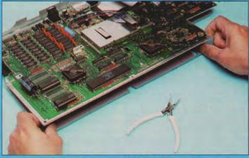
Carefully remove the motherboard from the base screen. Hold the board at the corners and push up with your fingers whilst holding the screen with your thumb.
