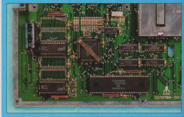
Remove the case, disk drive and power supply to reveal the motherboard as in the top picture. Then identify the 68000 processor, the GLUE chip, the existing TOS and the slots to be used for the upgrade.
