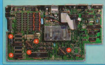
1. 68000 Main processor chip. ● 2. Existing TOS1.02 chips. ● 3. Spare slots used for new TOS. ● 4. MMU chip. ● 5. Glue chip.
