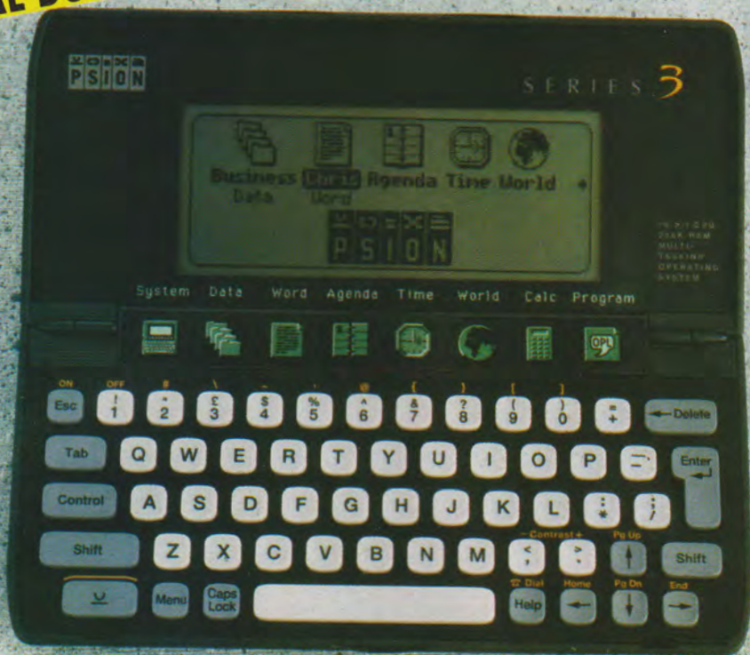
The Psion Series 3 organiser has Word and a spreadsheet built in. It also features a complete programming language.
