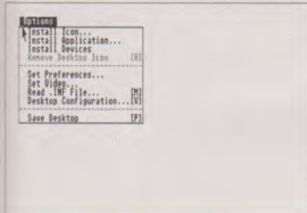
Menu entries now have keyboard equivalents (which are shown after the item) for direct selection from just a single key stroke.
