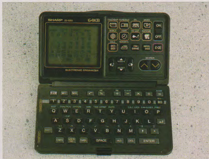
The ZQ-5200 has most of the functions of the older IQ-7000, but without the expansion card feature.
