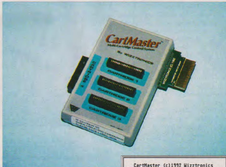
The CartMaster desk accessory or program lets you select which of the four cartridge slots is active.
