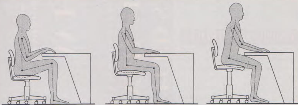
The middle picture shows how you should sit to reduce the likelihood of back problems. On the left you are too low and on the right too high.
