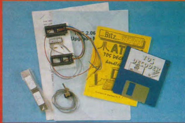
Left: Analogic Bitz board to add the new TOS to STFM or STE
