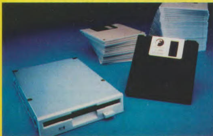
The floptical drive and disk. Will also read and write D/S and HD disks.
