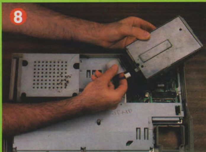
8 Unplug both of these. The smaller cable supplies power and is a bit awkward to remove; it will come free after a bit of wiggling. The 34-pin ribbon connector pulls straight off.
