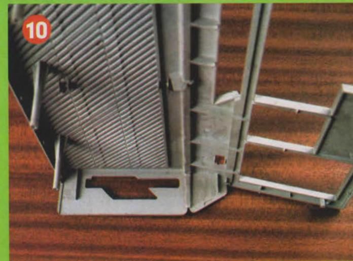
10 Cut horizontally along from the bottom edge of the drive eject button opening and vertically down at the sides. This should give you .....
