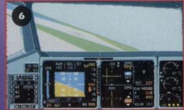
6 ● Turning onto the final approach – the ILS bars in the centre of the cockpit should cross in the middle
