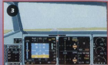
3 ● Power up to 100 per cent and lift the nose up once the speed reaches about 145 knots
