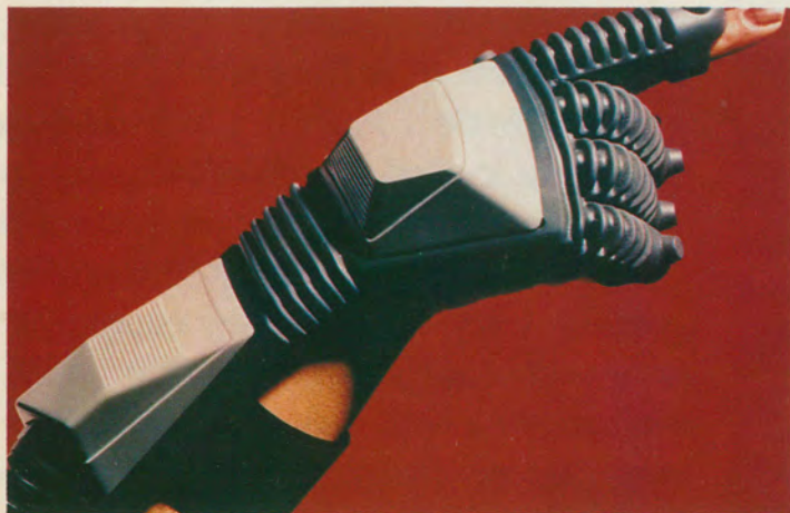
This is the Data Glove, which can be used to pick up and move objects around.
