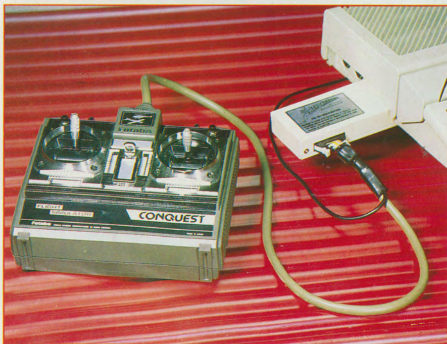
The kit comprises a Futaba R.C. unit, single cartridge and it doesn't have the usual plate of spaghetti usually associated with add-ons.
