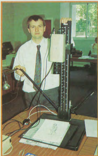
▲ John Prince demonstrating the RGB image process. Using a video camera, the team can capture hand-drawn graphics and spin an RGB wheel to get the colour.
