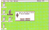
Early STes eat hard disks (or at least, they corrupt the data on them) and the required modification can be expensive.
