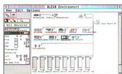
As you link "virtual" equipment in Notator Logic's Environment page you create MIDI Thru facilities automatically.
