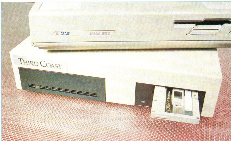
The TCT Tape Streamer uses a standard casing. With this version, the Streamer is built in to the same box as the hard disk unit.
