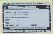
Records can be displayed either as lists or as page forms. Note the Forward, Stop, Backward and Print buttons on the form, and that there is no Fast Forward, video-style, as in Superbase. For elementary functions such as entering, erasing, editing and searching for records, alternatives to the dropdown menus are provided by the function keys and the row of First Word Plus lookalike buttons at the bottom of the screen.
