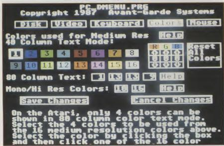
The pc-ditto configuration program allows many of the ST's facilities to be used by the emulator.
