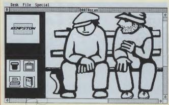
The software itself is very easy to drive. This shot shows simple black and white line art scanned at 200 dpi. Underneath the Kempston logo are the four main functions which are also available from the pull-down menu. They include: scan; print; disk operations; and quit. To start, you must also press the 'scan' button on the scanner's hand grip.
