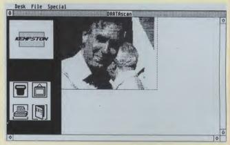
In some cases, not every detail needs to be retained from the original. Here, we have banded the face of the individual, and saved the block to disk. The saved block has then been loaded back into the work screen. The normal 'SAVE' routines will identify a cut block automatically.
