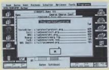
Access to a wordprocessor (for mailmerge and report forms), the INIT, DRC, REORG modules, the TALK programming environment and a command line interpreter from within Adimens are possible through the Programs menu. Paths can be defined in this dialog box and saved to a configuration file. Although this facility is only really useful for two-disk or hard disk setups, Adimens will happily work on unexpanded, single-drive 520STs.
