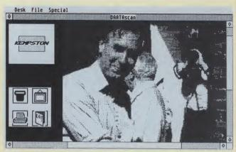
How well does the scanner handle a colour photograph? Quite well, given the sixteen grey levels. This photo was scanned using setting one of the dither routines. Careful adjustment of the contrast control would add some further detail to those areas which have become blocked out.
