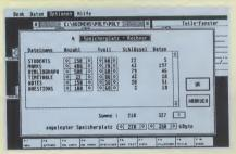
Adimens needs to reserve disk space for the data and index files, but compresses these to optimise disk utilisation. Still in INIT.PRG, this screenshot shows the large dialog box requiring the user to indicate the expected maximum record numbers and anticipated average field space usage. All these values can be modified later if, as is usually the case, existing data files are outgrown in practical use.
