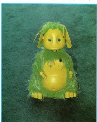
light; touch and others. The genuine working model is completely self-contained, crammed full of electronics with 4 PCBs inside it, 13 batteries and about 48K of optimised C and machine code software.
