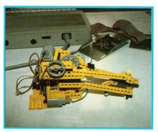
Lego motors, bi-directionally, or eight uni-directionally. The board can drive up to 3 amps, so solenoids could even be used. There is no software support for stepper motors, preferring to adopt the cheaper and more flexible DC motor plus shaft-encoder principle. There are also up to eight outputs to drive Futaba servo motors. The inputs can be TTL inputs or switch closures. Included is the ability to drive two of the new Lego shaftencoders.
