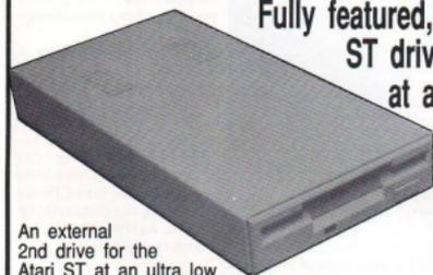
An external 2nd drive for the Atari ST at an ultra low price - complete with its own plug-in external power supply! Based around a top quality Citizen drive mechanism, this drive gives the full 720K formatted capacity. Quiet in operation, neat slimline design, colour matched to the ST, with a long connection cable for location left or right of the computer.
