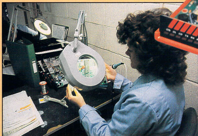
Making the MicroLink multi-speed modem: The task involves more than 200 components requiring 600 soldered joints – every one of them inspected at least once. The device is built around the new K222 V21/22 chip from the US which is much more reliable and easier to interface than the old 7910 V21/V23 chip. Only after two full-function tests – interposed by a 24-hour soak test to burn in the components – is the MicroLink modem ready for the customer.
